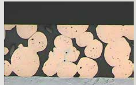
Fig. 8: Condition of sliding surface during service life
