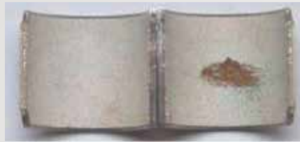
Fig. 35: Local damage caused by cavitation
