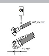
Coat the thread of the pipe socket with oil or grease.
