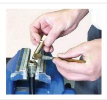
Hold the Ferrule with an SW12 hex driver and screw the SW10 standpipe clockwise into the screw sleeve.
