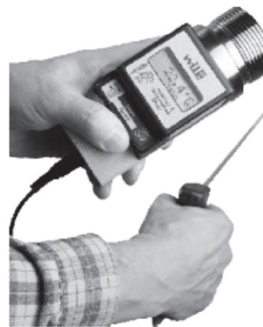
Wile-651 plugged in Wile-65 measures the temperature of stored grain, hay, compost etc. between 0-60°C
