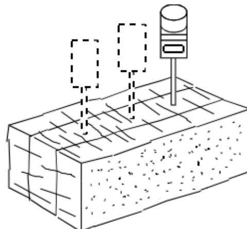
In round bales the moisture should be measured from several points around the bale.
