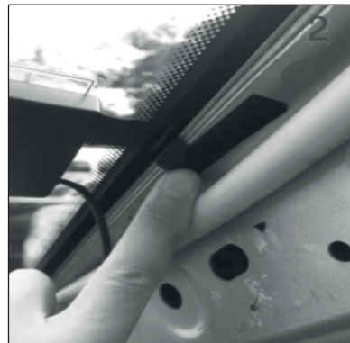
Stick the transparent part of the antenna on the windshield and put the black part (magnetic) on the metal frame.
