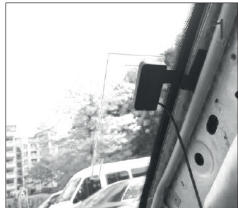
Stick the transparent part of the antenna on the windshield and put the black part (magnetic) on the metal frame.
