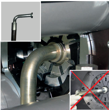
The S4 series can be used to crimp short 90° elbows fittings with along drop. This is impossible for other conventional machines.
