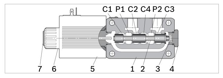
A valve basically consists of a housing (1), a control spool (2), a return spring (3) and a solenoid (5). It is designed to connect two inlet lines P1 - P2 (normally a set of hoses) and divert them to either the outlet ports (C1 - C4) with spool in position "0", when the solenoid is de-energized, or to the outlet ports (C2 - C3) with spool in position "1", when the solenoid is energized.
