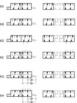
1) Minimum pressure 4 bar (58psi) with external drain (E), maximum pressure 200 bar (2901psi). With internal drain (I), at the minimum pressure (4 bar - 58psi), add the working pressure with ratio of 6,5:1. Example: With working pressure 100 bar (1450psi), minimum pilot pressure is 19.38 bar (281psi) ((100:6,5) + 4 bar (58psi)).
