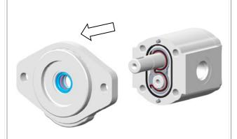
Remove the front pressure plate and the gears.
