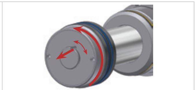
Fig. 7 Remove securing bolt/Screw piston loose
