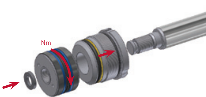
Fig. 9 Mounting cylinder Bore 40 up to 100
