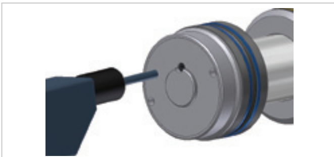
Fig. 6 Bore out securing bolt
