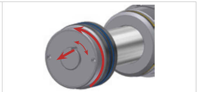
Fig. 7 Remove securing bolt/Screw piston loose
