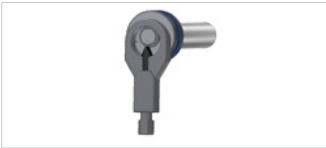
Fig. 4 Cleave open crimp ring
