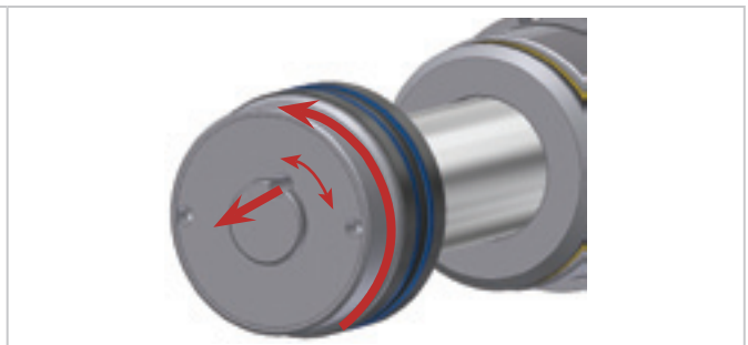
Fig. 7 Remove securing bolt/Screw piston loose
