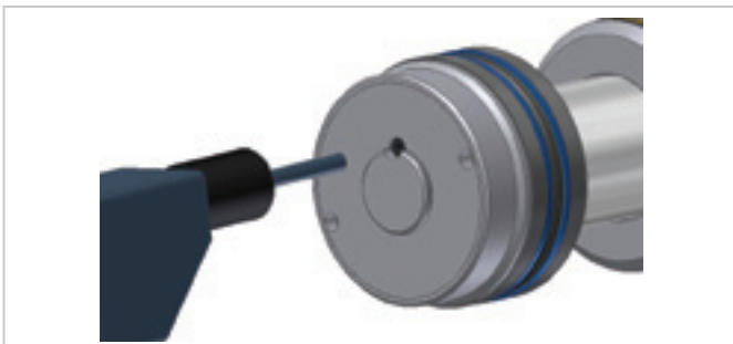
Fig. 6 Bore out securing bolt
