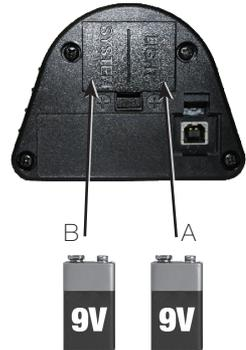
NOTE: When you first turn on the tester if the system battery is at or below 5% the tester will automatically flash the battery life on the display to let you know the battery needs to be replaced. If the backlight battery is fresh and the system battery needs replacing, the backlight battery can be used to operate the system by moving it to the system battery location.
