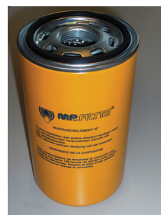
Fig. 9: Oil filter element to be replaced
