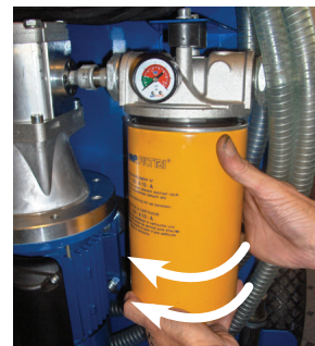
Fig. 6: Loosen the filter by turning it counterclockwise
