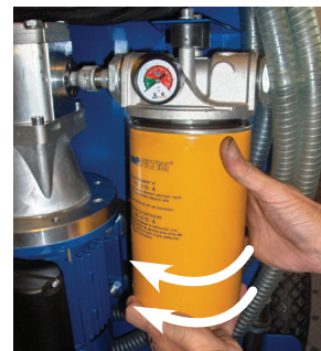
Fig. 6: Loosen the filter by turning it counterclockwise
