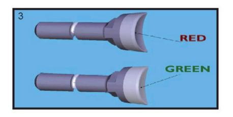
3) Because soil conditions vary, we offer our carbide tips in two different styles. Red and Green. The Red carbide tip has a deep dish, cuts fast, and works well in cleaner soils. The Green carbide tip, though still fast cutting has a shallow dish and is designed for tougher and more unpredictable soil conditions.
