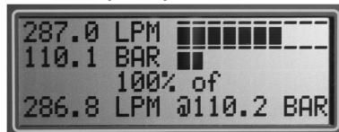
This screen is used for testing pump volumetric efficiency. The screen initially displays flow and pressure on the top two lines as in SCREEN 2 and power on the bottom two lines. Once the efficiency reference point has been captured, then the third line displays the current efficiency and the bottom line shows the reference point, the top two lines will continue to display the current flow and pressure.
