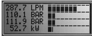
This screen displays the measurements in the same order as in SCREEN 1, but this time displays the value, engineering units and a bar graph which corresponds to the value indicated. The bar graph is scaled from zero to the maximum value for the tester (see below). Bottom line displays Power or Temperature depending on selection.
