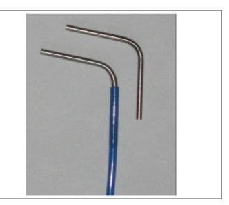
Open the CFC hose switch off (KFC.001.TR/TL) and insert the filling tube. Make sure that the filling tube is in the recess intended for it in the hose switch off.
