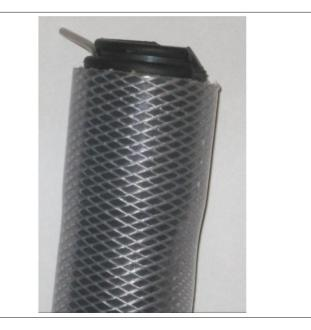
Mark a distance of 40 mm on the distributors tube of the distributor to which the hose switch off will be installed.
