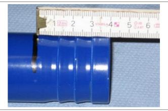
Generously lubricate the marked section of the distributor tube.
