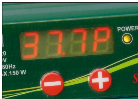
Display with temperature in Programme Mode (temperature followed by "P")
