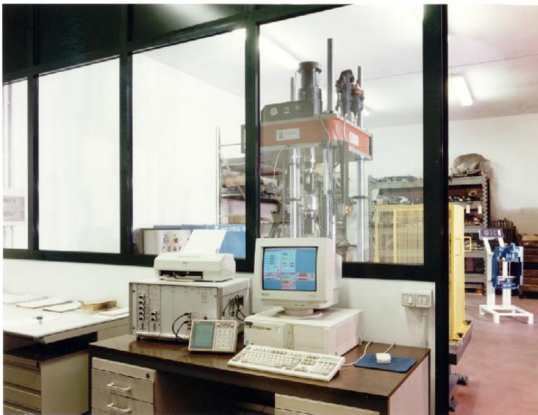
Test Bench for dynamic stress tests – Resistance tests
