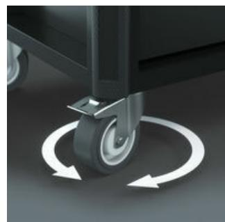
The two swivel castors are equipped with a double stop: The locked castor reliably prevents it from rolling away, the locked spindle carrier prevents the castors from turning unintentionally, e.g. on sloped surfaces. The oil- and acid-resistant elastic wheels ensure smooth running. A protective ring prevents the ingress of dirt and threads.
