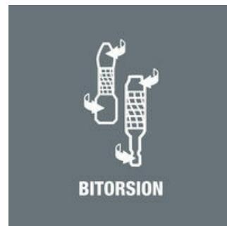
Peak forces that occur in power tool applications often result in premature wear of bits or damage to the screw head. This usually occurs during initial power-up and when the screw comes to a standstill. Screwdriving could become more productive and safer if these peak loads could be minimised. The Wera BiTorsion system prevents premature wear. The service life of the tool is extended and the productivity of power tool applications significantly increased.
