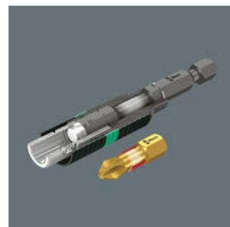
The optimally coordinated features of the torsion zones on the bit and holder permit a phased yield when under strain. The two-phase system prevents premature wear. Moreover, a long tool service life is also ensured by the hardness of the bits that matches the respective application.
