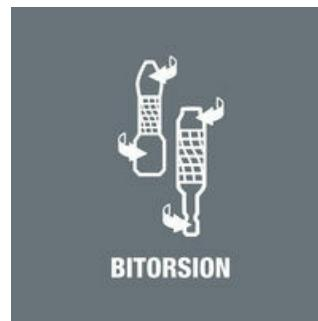
Peak forces that occur in power tool applications often result in premature wear of bits or damage to the screw head. This usually occurs during initial power-up and the when the screw comes to a standstill. Screwdriving could become more productive and safer if these peak loads could be minimised. The Wera BiTorsion system prevents premature wear. The service life of the tool is extended and the productivity of power tool applications significantly increased.
