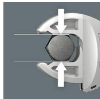
The parallel smooth jaws of the Joker 6004 allow surface pressure and can thus prevent rounding of the bolt or screw head, which can occur during power transmission on corners.
